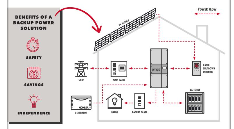
As solar energy is generated it is used to power your home in place of electricity from the grid. Any electricity generated in excess of what you use can be stored in the battery for use during peak rate times, Public Safety Power Shutoff or other outage.
