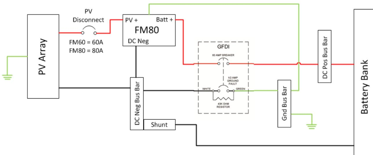
Figure 1 - FM80 Standard GFDI Wiring
