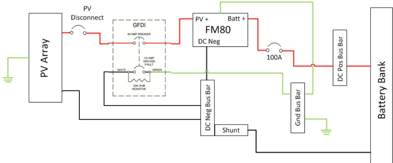
Figure 2 - FM80 Extended Performance GFDI Wiring
