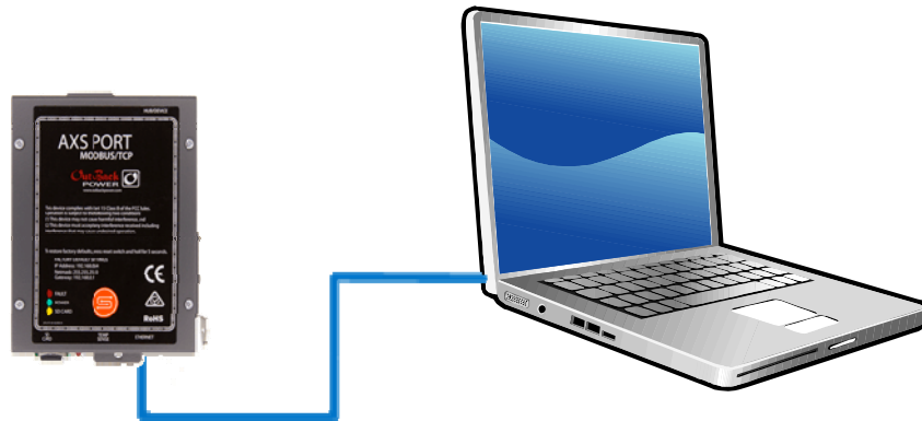
Figure 1: AXS Port without router
