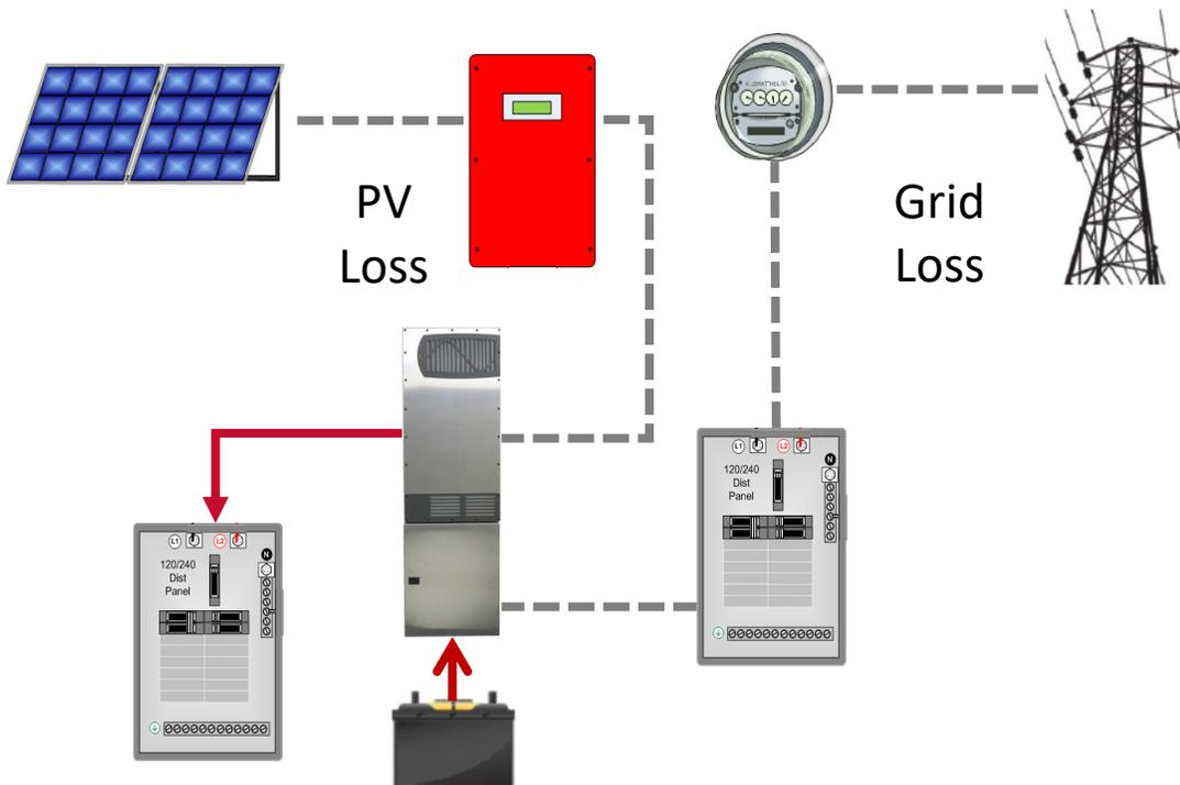
**Figure 5 – Off-grid current flow due to PV loss or GDI power overcharging battery bank**
