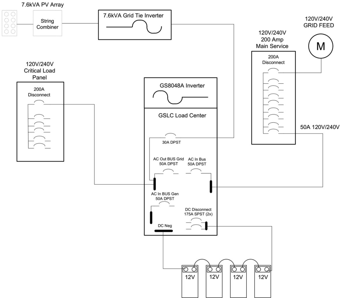
Figure 6 – Single line diagram of GDI inverter connection to Radian inverter
