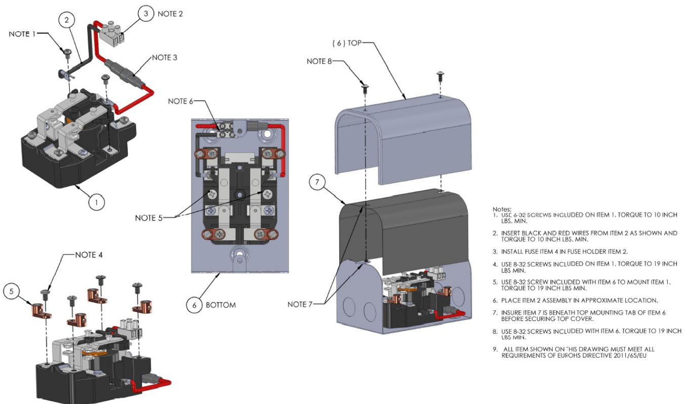
Figure 7 – GS-AC-GEN-KIT, Generator Protection Relay from OutBack
