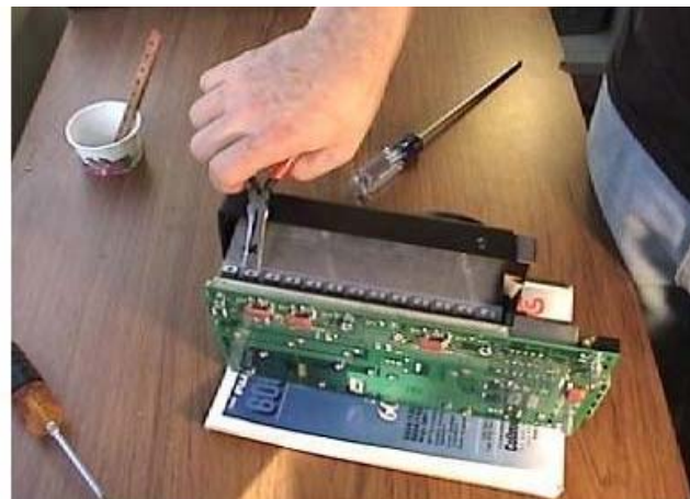
Figure 7b Loosening the MOSFET with needle nose pliers
