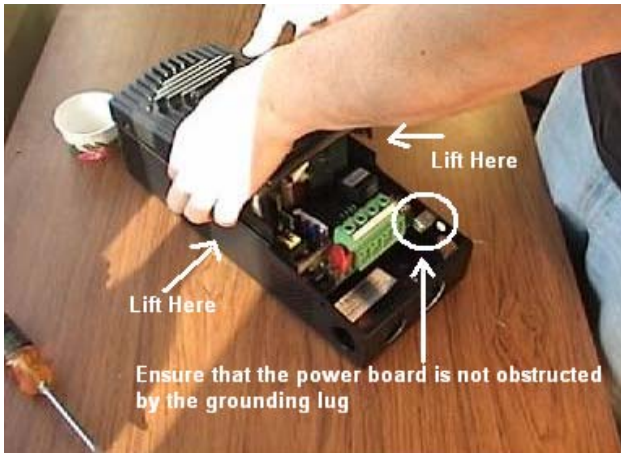
Figure 5a Heat sink removal procedure
