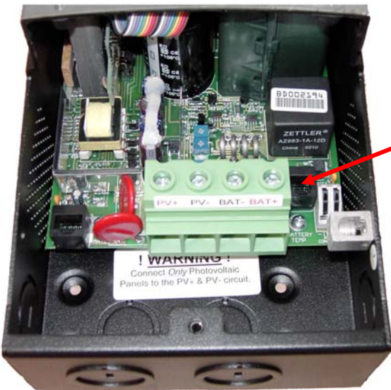
Figure 22 Battery temperature sensor jack location
