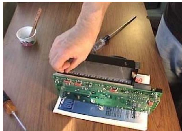
Figure 7a Freeing the MOSFET from the insulator
