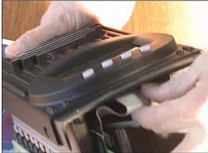
Figure 17 Gently pulling on the ribbon cable
