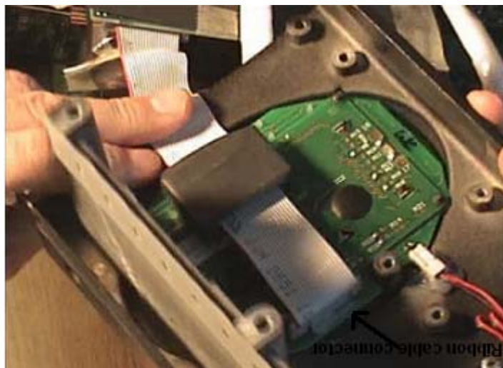
Figure 16 Ribbon cable connector over the LCD
