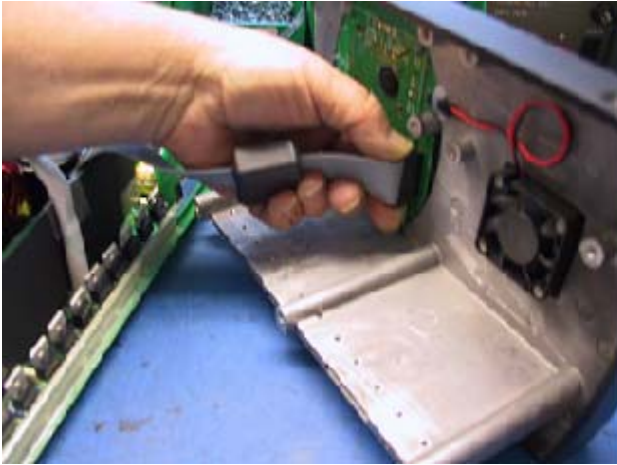
Figure 11a Ribbon cable removal
