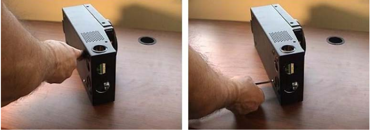
Figure 2 Back screw removal
