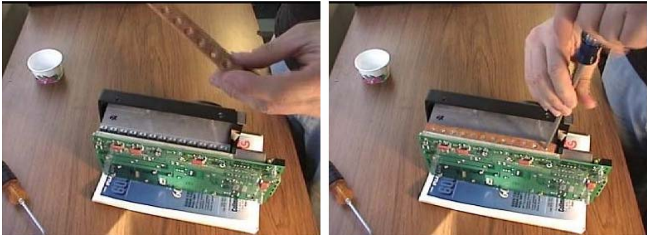
Figure 19 Installing and tightening the FET mounting screws
