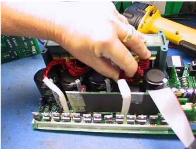
Figure 12 Orientation of inductor wires.
