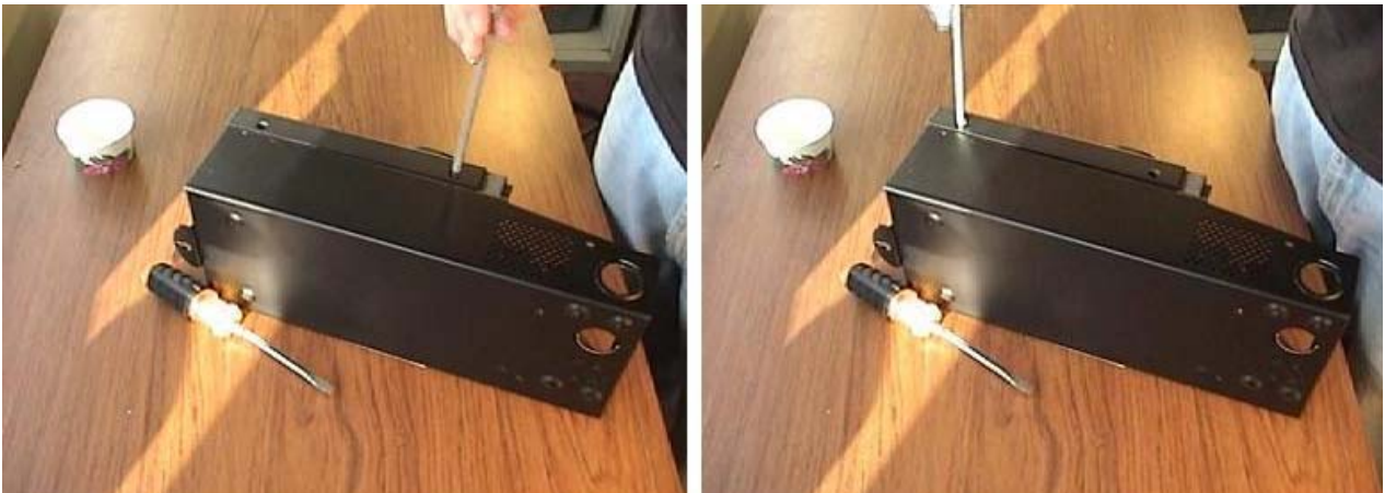
Figure 3 Side screw removal
