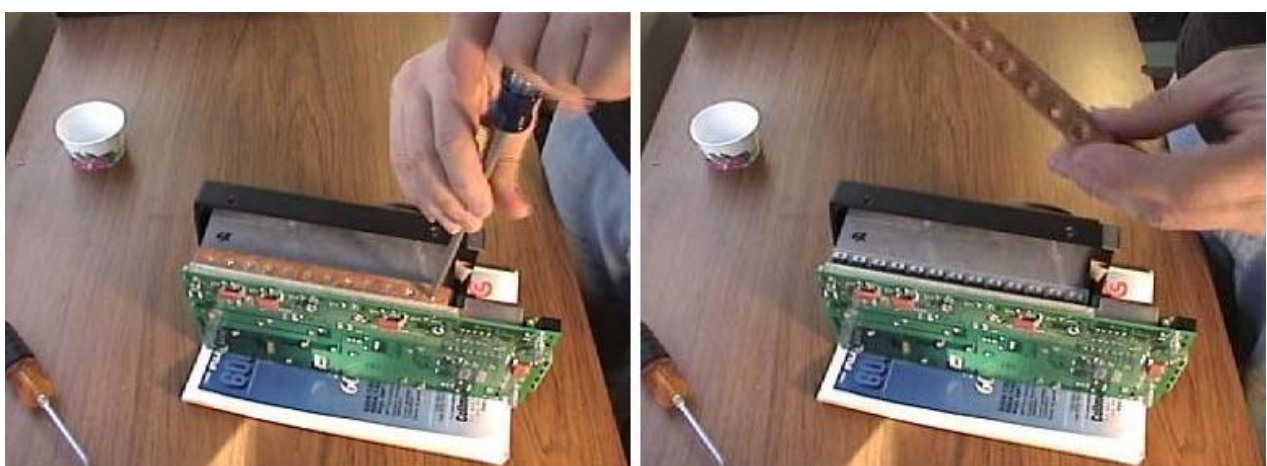
Figure 6. FET bar removal procedure
