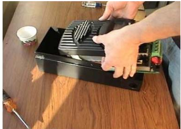
Figure 5b Sliding the heat sink off the chassis
