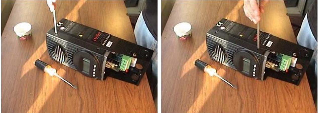
Figure 4 Side screw removal
