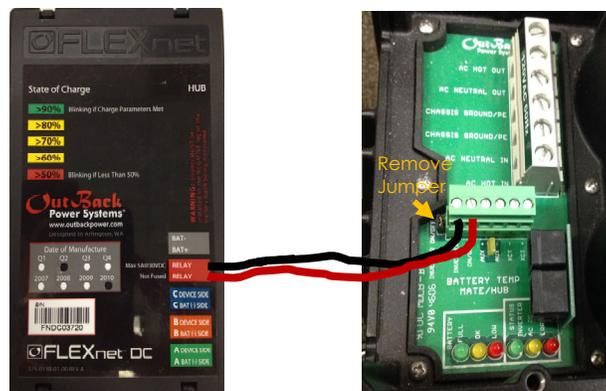
Figure 2 - how to prevent dead battery condition
